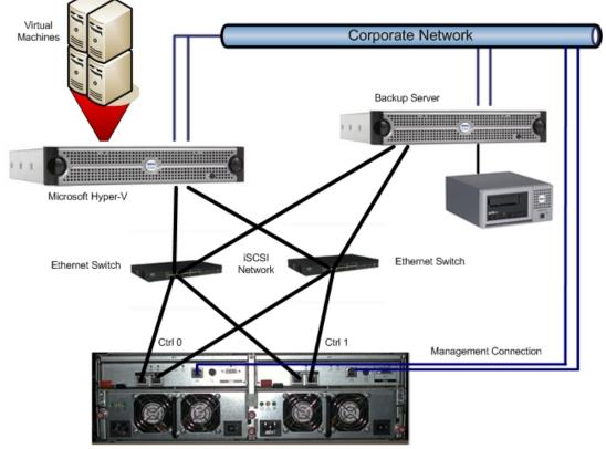
Figure 2 DELL PowerVault MD3000i (IP-SAN)
